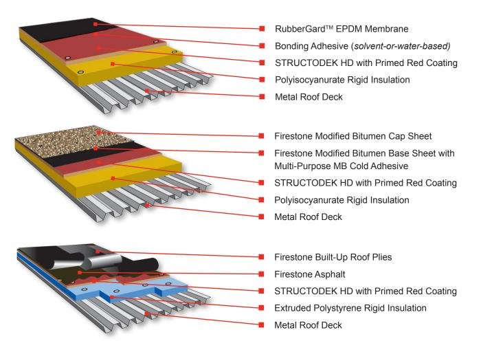
Note: STRUCTODEK High Density Fiberboard Roof Insulation should not be installed in moist environments and must be kept dry prior to and during installation. The material is combustible and must not be exposed to open flame or excessive heat.
